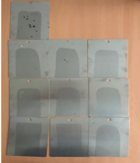
Picture 1: at the top: without additive left: SCHWEGO flash inhibitor EL 1320 middle: SCHWEGO flash inhibitor EL 1420 right: SCHWEGO flash inhibitor EL 1520
